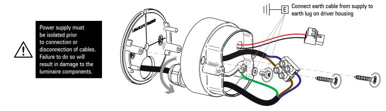
Connect the luminaire to the driver using the connector. Then screw the luminaire body
