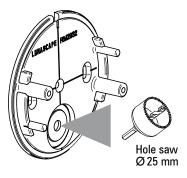
Pull the supply cable through the gland hole and screw the mounting back plate to the mounting surface ensuring the back plate is level and in the correct orientation for the luminaire you are wanting to install.
