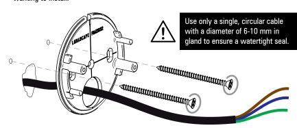
3. Screw the gland into the back of the driver housing ensuring the o-ring is in place between the two components.
