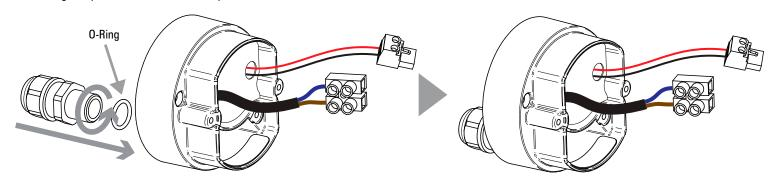
Pull supply cable through gland and tighten up as shown. Connect the supply cable to the driver using the terminal block. Do not forget to connect the earth wire from the supply cable to the earth lug on the driver housing. Screw the driver housing to the mounting back plate.
