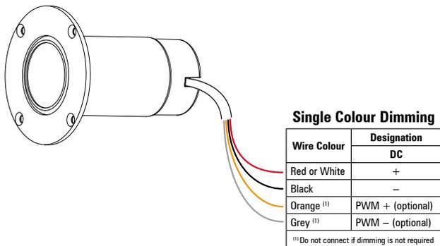
**NOTE:** If dimming is required use LS6125 PWM to 0-10V dimming.
