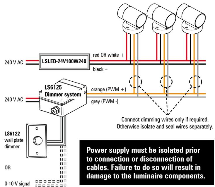
**Power supply must be isolated prior to connection or disconnection of cables. Failure to do so will result in damage to the luminaire components.**
