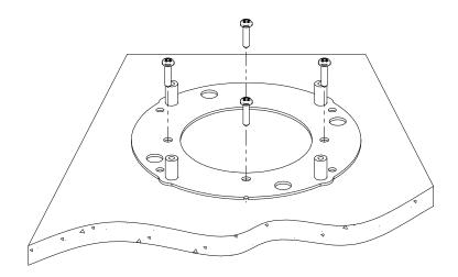
**Step 2** Align luminaire with the pre-install plate; tighten screw to secure luminaire to pre-install plate.
