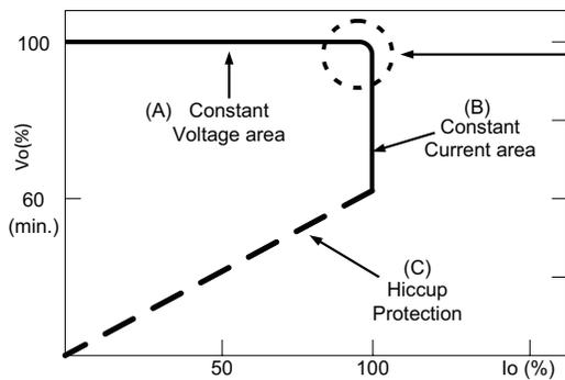
In the constant current region, the highest voltage at the output of the driver depends on the configuration of the end systems. Should there be any compatibility issues, please contact MEAN WELL.
