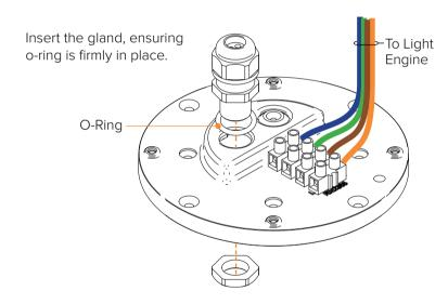
Feed supply cable through gland and tighten. Outer diameter of cable should be Ø5-10mm. Connect supply cable to terminal block.
