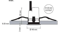
Fold legs up on the ceiling clip and insert into hole and feed LS9404LED cable through mounting clip.
