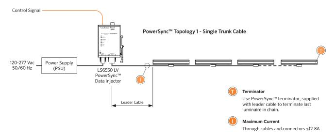
Up to 24 luminaires per 48V PowerSync circuit / LS6550 Low Voltage PowerSync Injector
